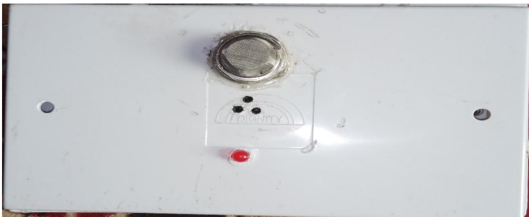
Figure 4.8 complete gas leakage detector device ready and encased in a parterres
