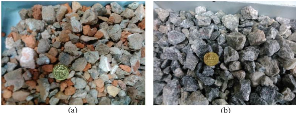
Fig. 4: (a) Recycled Construction and Demolition Aggregates; (b) Natural Aggregates (Jayakody et al, 2018).
