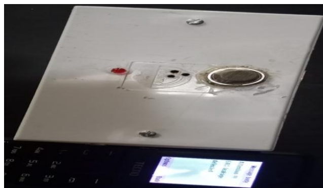
Figure 4.9 functional gas detector with mobile phone receiving short messages service signal via GSM module
